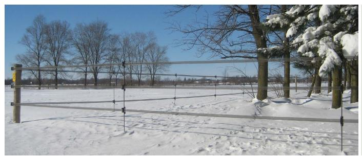
HorseGuard fiberglass posts are 5.57 ft. /1.70 m. and should be sunk 15 in. /40 cm. into the ground. With a diameter of /0.47"/12 mm. they are essentially unbreakable, rot-proof, rust-proof and twist resistant, nearly indestructible. Their function is to hold the tape inside the insulators at the right height on the line.
