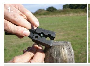
1. Put the end of the cable into the hole marked "strip"
