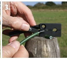
**3.** Without opening the crimper, pull the cable to strip it
